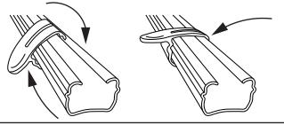
Always rotate the slats to the "open" horizontal position before raising or lowering. This assures smooth operation and increases the life of the blind.
